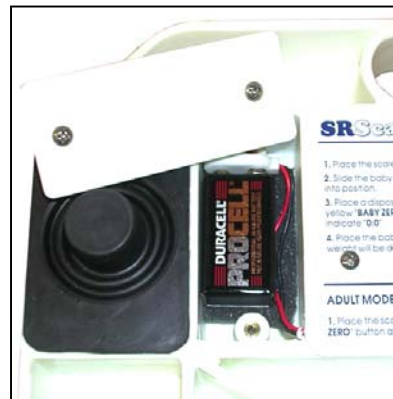
Figure 3: SR241/SR241SO Battery Compartment
